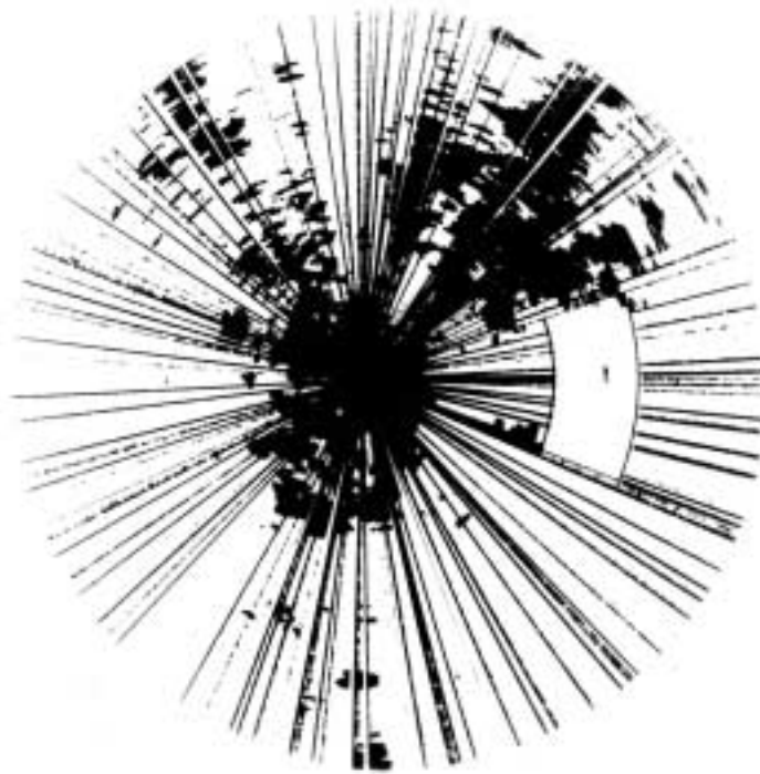
Figure 2: Adaptive suppression of simulated weather clutter
